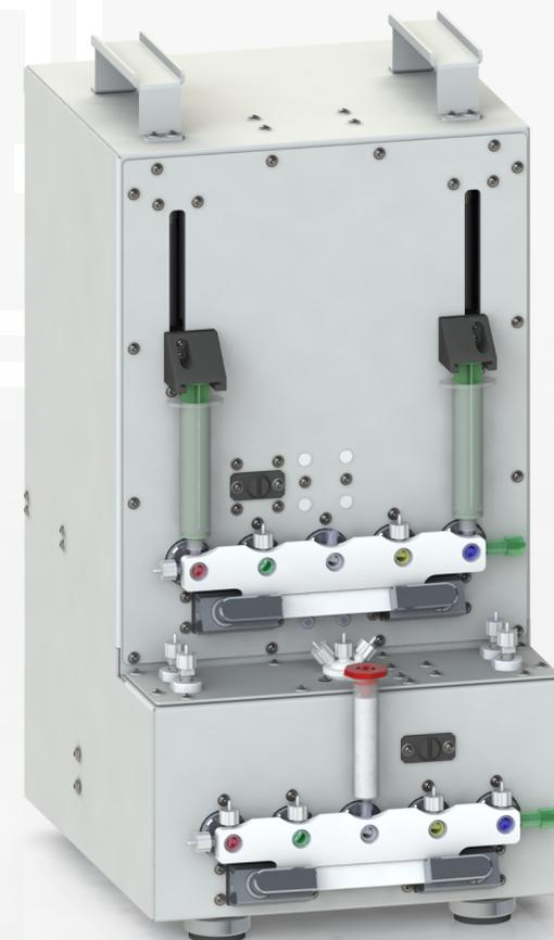
The reagent distribution subsystem is based on the use of two blocks of rotary valves (a total of 10 valves). The liquid transfer lines are all fully disposable (blocks of rotary valves, reaction vessel, transfer lines and connections). The device is equipped with compact built-in syringe pumps with adjustable elution rate.
